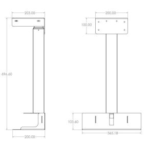
Height: Closed 69.6cm Open position 135.6cm Width: 36.5 cm Depth: 20 cm
